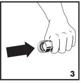
3. Visually inspect the fitting to ensure the grip ring, separator ring, and seal are in place, clean and free of contaminants. Only original NIBCO<sup>®</sup> yellow HNBR BenchPressG<sup>™</sup> seals are to be used.
