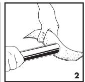
2. Prep pipe to a smooth and even surface with a fine arit sandpaper. The surface should be free of indentations, oil, and debris. Do not use engraved or stamped pipe. Indentations in the pipe may result in an improper seal. To avoid damage to the O-ring, the pipe must be free of burrs and sharp edges.
